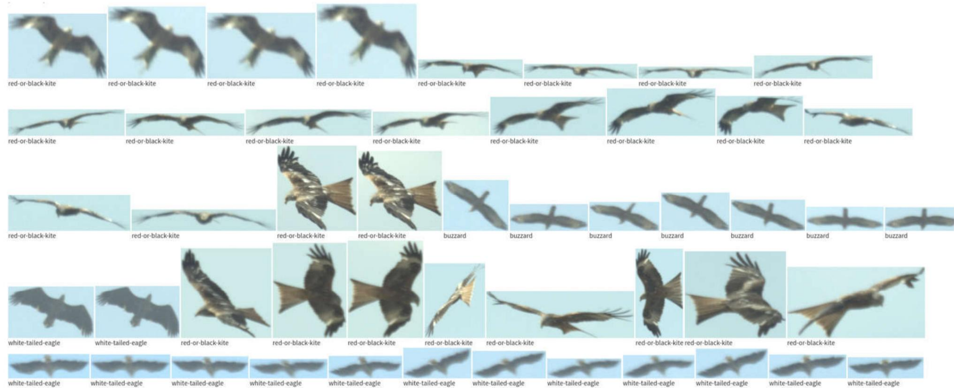
Figure 62: Sample images with the original classification by IDF. Version 2 of the neural network. The three different bird species are correctly identified by IDF. In software version 2, there is no longer a distinction between red and black kites, they form a category. Location Bütow, June 17th, 2020.
