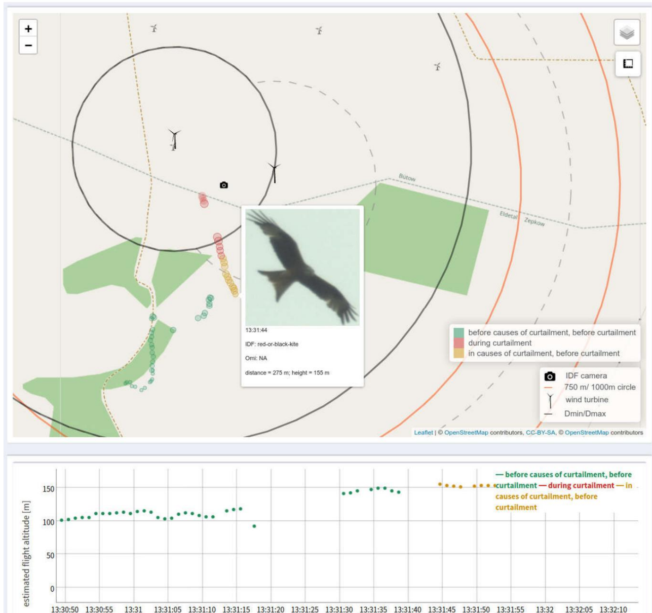
Figure 66: Shutdown when entering the inner spacer cylinder (inner black line) of the western wind turbine at the Bütow site. The shutdown for this wind turbine (red dots) was triggered a few seconds after the shutdown for the eastern wind turbine (see Figure 65). Location Bütow, May 18, 2020.
